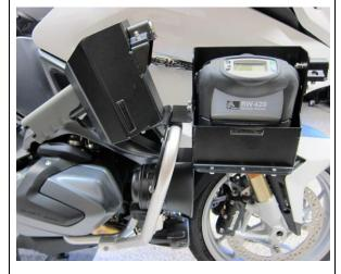
**Forward High Mount:** FMS Accessory Zebra printer boxes are made from powder-coated heavy duty aluminum to resist corrosion. The mounting brackets are produced from powder-coated steel and are connected via five bolts. This does enable the case to be replaced in the event it becomes damaged. Attach the provided Velcro to the printer and the box to secure the printer from vibration / damage.
