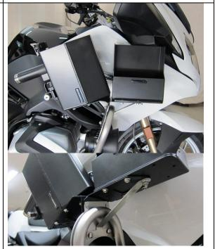
**Rear Mount:** FMS Accessory Zebra printer boxes are made from powder-coated heavy duty aluminum to resist corrosion. The mounting brackets are produced from powder-coated steel and are connected via five bolts. This does enable the case to be replaced in the event it becomes damaged. Attach the provided Velcro to the printer and the box to secure the printer from vibration / damage.
